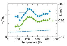
Fig. 4. Temperature dependence of the Fermi energy (green + symbols, right ordinate, the zero referring to the top of the valence band) and of the density of states effective mass (blue dots, left ordinate) of  $Tl_{0.02}Pb_{0.98}$ Te compared to that of Na-PbTe (blue dashed line).
